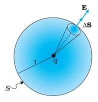
The figure shows a sphere of radius r, which encloses a point charge q at its center.  $\Delta S$ , is a small area element.
