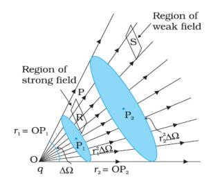
This means that if we place a small planar element of area  $\Delta S$  normal to E, at a point, the number of field lines crossing it is proportional to E  $\Delta S$ .
